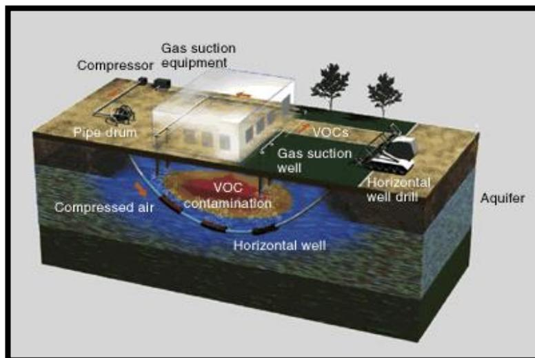
In a horizontal system, the bore acts as both the recovery and transfer line. The same pipe provides both the screened section to extract vapors and a blank section to carry the vapors back to the surface and then to a recovery area to be processed. If numerous areas are affected the pipes can be tied in to a common collection area.
